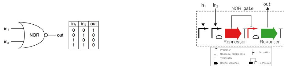
Fig. 1: Logic and Genetic NOR Gates
